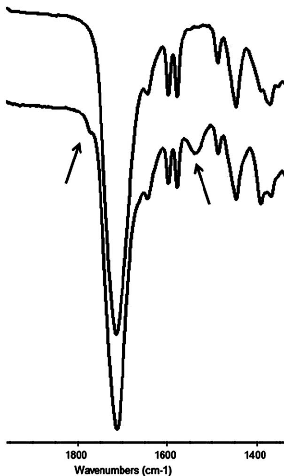
Figure 5 FTIR spectra of unmodified and chain extended UPEs.
